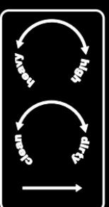
**heavy - high:** This is the filter knob. Heavy is a deep bass booster and high is a treble screamer. Turning the knob sweeps through a wide range of cut and boosted frequencies.
